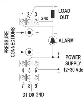
Figure 5 – Electrical connections
