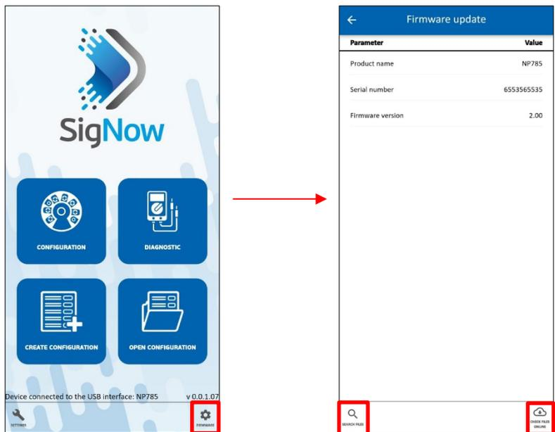
Figure 23 – Upgrading firmware via app
